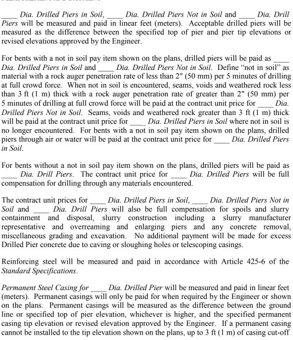
will be paid at the contract unit price for *Permanent Steel Casing for \_\_\_\_ Dia. Drilled Pier.*
